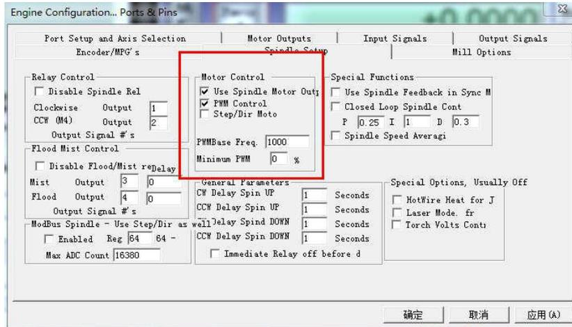
Enable spindle output. as shown below:
